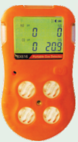
PORTABLE MULTIGAS DETECTOR (LEL/HS/NH 3 /O 2 ) MODEL - BX616
